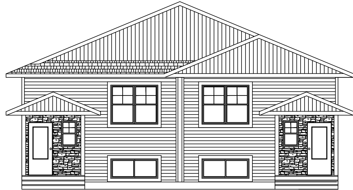
FRONT EXTERIOR ELEVATION
