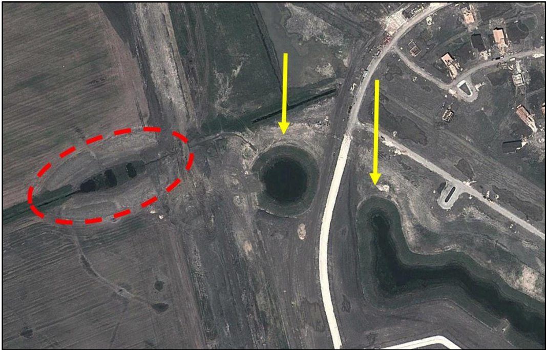
Figure 6.3. Sedimentation pond (indicated by dashed red oval) installed as a temporary sediment control measure upstream of an NSP network (indicated by yellow arrows) during the construction phase.
